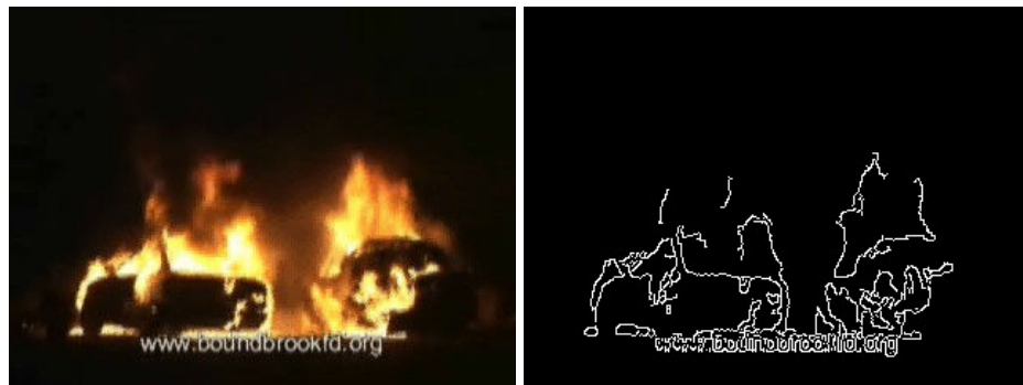
Figure 3-3. Canny Edge detection is used for finding contours
